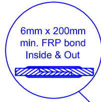
SECTION-JOINT DETAIL
