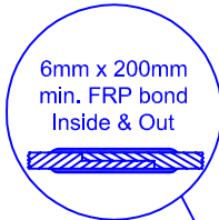
SECTION-JOINT DETAIL
