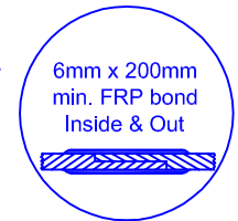
SECTION-JOINT DETAIL
